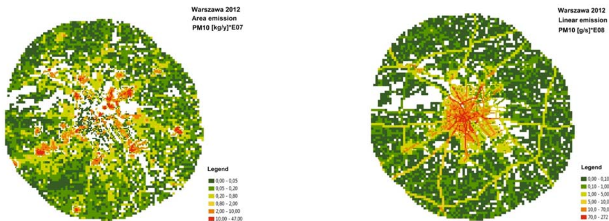
Fig. 2. The PM_{10} emission fields for the area sources (top) and the line sources (bottom)
