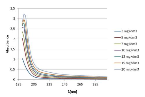
Fig. 2. Typical UV absorption spectra of FA separated from treated wastewater in Plaszów plant
