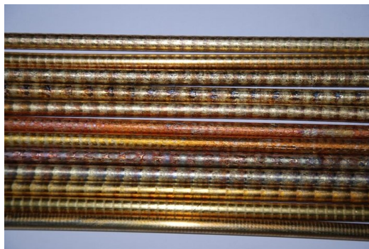
Fig. 4. CuZn39Pb2 alloy continuous castings where the order: bottom – casting no 1. top – casting no 12 is preserved
