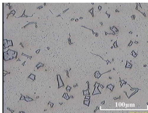
Fig. 4. Microstructure of cast steel (0.8% C, 16% Mn, 1.4% Cr, 2% Ti) after solution heat treatment; austenitic matrix with primary titanium carbides uniformly distributed in this matrix; nital etching [1]
