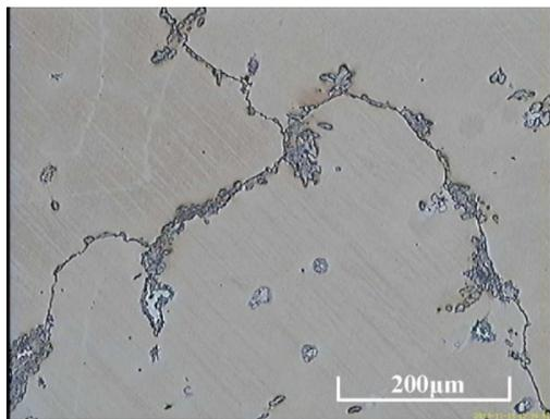
Fig. 1. As-cast microstructure of Hadfield steel; austenitic matrix with precipitates of alloyed cementite; nital etching [1]
