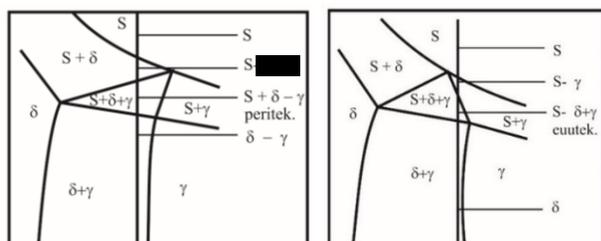
Fig. 1. Solidification of the austenitic steels depending on peritectic reaction
