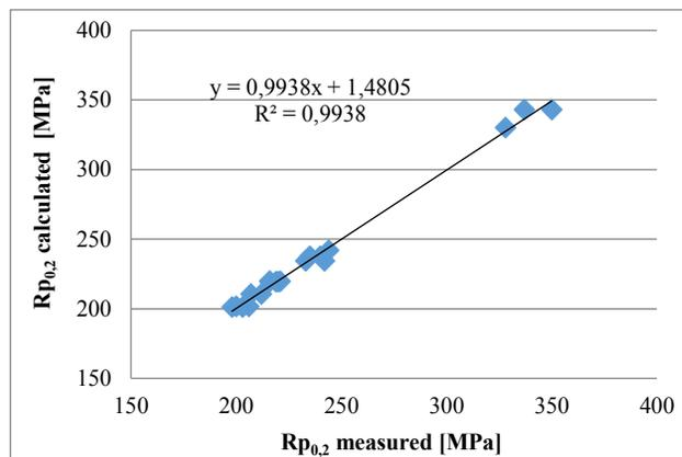
Fig. 3. Matching the calculated and measured  $R_{p0.2}$  values
