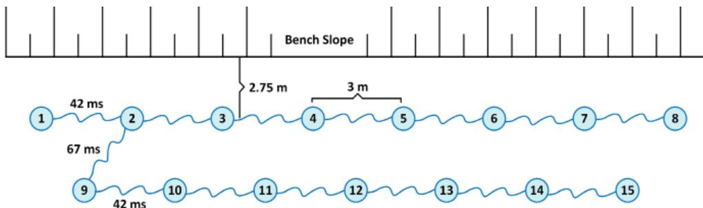
Fig. 6. The blast-hole design with 15 holes
