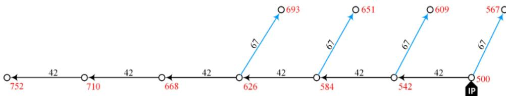
Fig. 10. Time-delays of the group-blast
