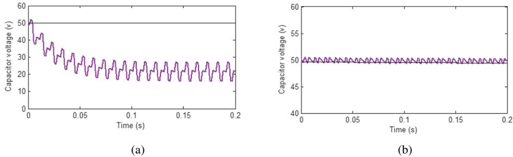
Fig. 7. Capacitor voltage  $V_c$ : (a) based on ECSA; (b) based on N-R algorithm
