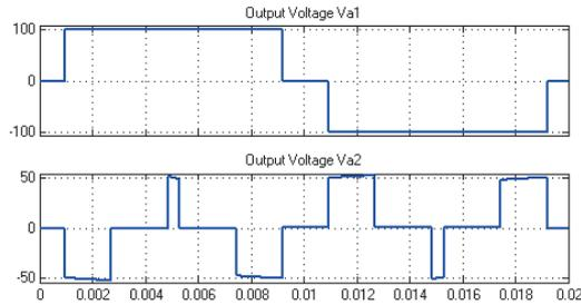
Fig. 10. Output voltage waveform for  $V_{a1}$  and  $V_{a2}$
