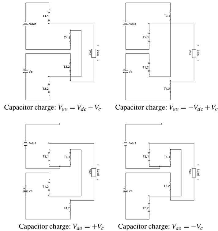
Fig. 2. Capacitor charge / discharge states
