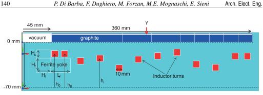
Fig. 1. Geometry and design variables of the induction heating benchmark
