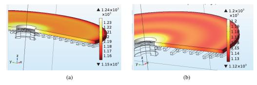
Fig. 8. Temperature distribution [°C] for the two end-points A (a) and B (b) of the front obtained by NSGA, shown in Fig. 7
