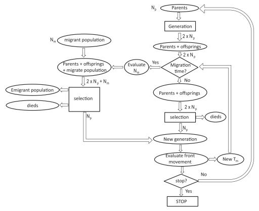
Fig. 6. Flow chart of autiomatic MNSGA algorithm
