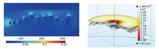
Fig. 4. Magnetic field [T] map (left), temperature [°C] field map (right)
