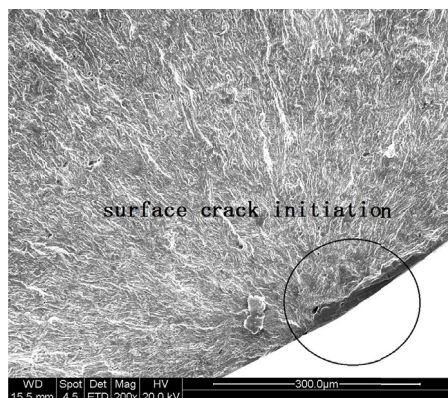
(a) Single crack initiation ( N_f = 1.76 \times 10^6 )
