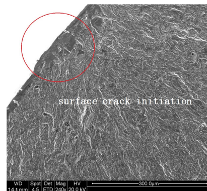
(b) Single crack initiation ( N_f = 7.12 \times 10^6 )
