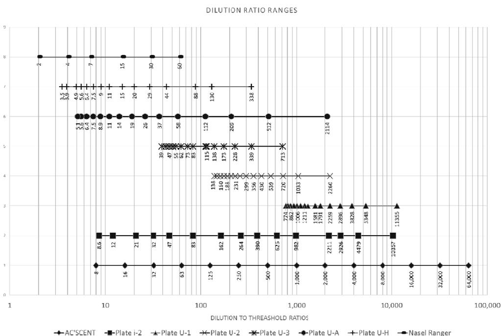
**Fig. 1.** Graphical representation of the range of the dilution ratios used by the AC'SCENT® International Olfactometer, the Nasal Ranger, and the different plates used by the Scentroid SM 100i Intelligent Personal Olfactometer. The x-axis, representing the dilution to threshold ratios, uses a logarithmic scale to display the data for a better visual comparison. This graph includes the values for each dilution ratio available (except the tightly packed data points for plates U-1, U-2, and U-3)
