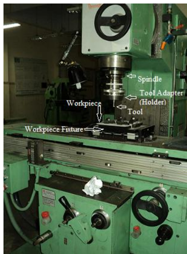
Fig. 2. FSW set up used for FSW experiments
