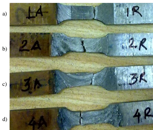
Fig. 4. Fracture location of the four samples
