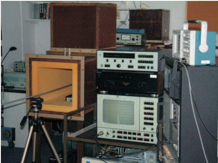
Fig. 3. View of a stand for testing active noise reduction methods.
