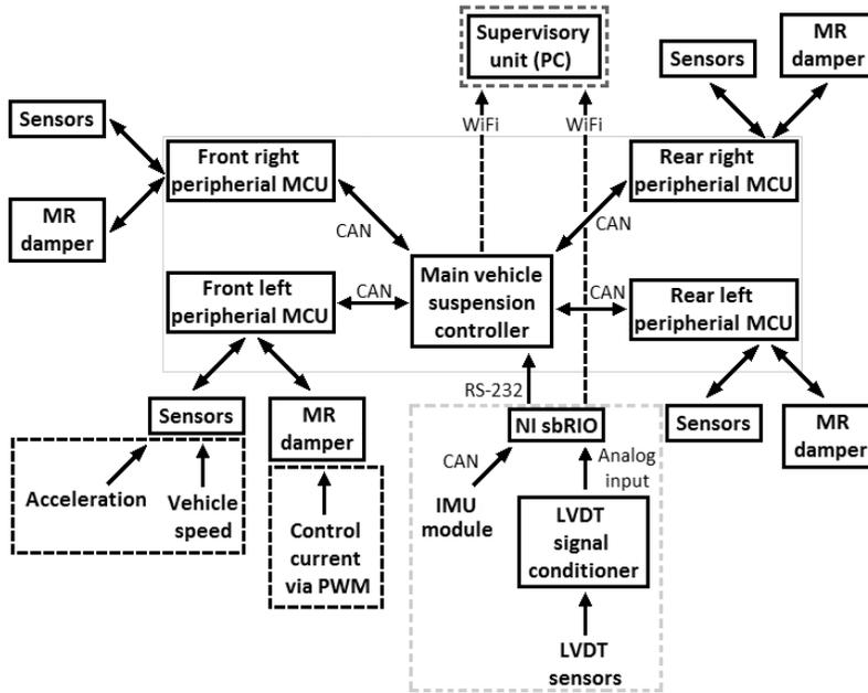
Figure 2: Architecture of the proposed measurement and control system
