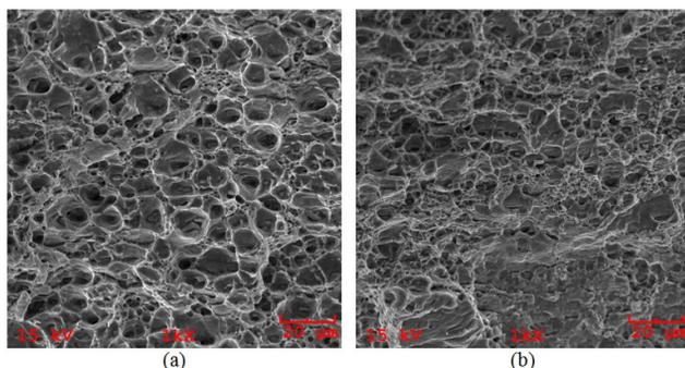
Fig. 7. SEM images of the fractured surfaces of extruded alloys, a) Alloy A, b) Alloy B
