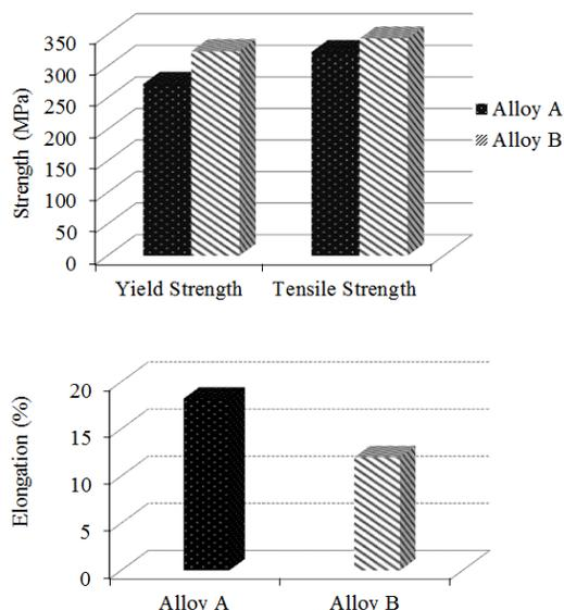
Fig. 5. Mechanical properties of the extruded alloys
