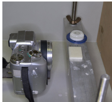
Fig. 1. Test bench for the measurements of the pattern's wetting angle
