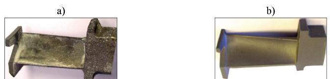
Fig. 5. Low-pressure turbine blade made of Ti-47Al-2W-0.5Si alloy after casting, knockout of the ceramic mould, cutting off the riser (a) and surface cleaning (b)
