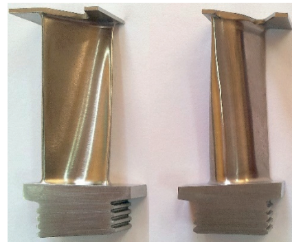
Fig. 10. Finished low-pressure turbine blades made of Ti-47Al-2W-0.5Si alloy
