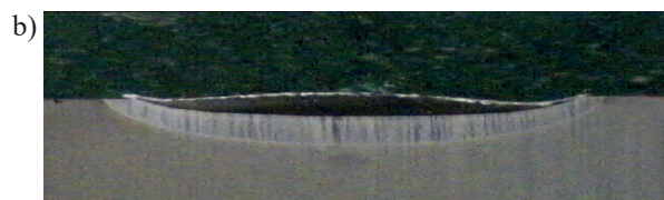
Fig. 6. The cross - section of laser surface alloyed 32CrMoV12-28 steel after laser alloying with a) WC powder and b) VC powder at laser beam power of 2.3 kW
