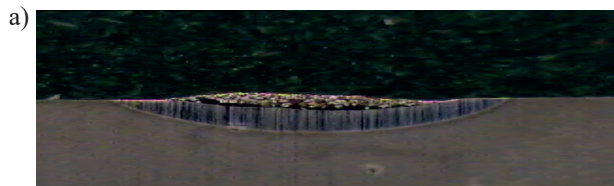
Fig. 5. The cross - section of laser surface alloyed X40CrMoV5-1 steel after laser alloying with a) WC powder and b) VC powder at laser beam power of 2.3 kW
