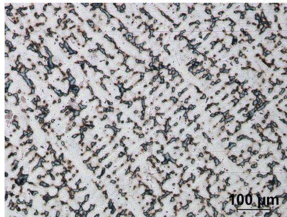
Fig. 2. Microstructure of cast Cu-3Ti alloy
