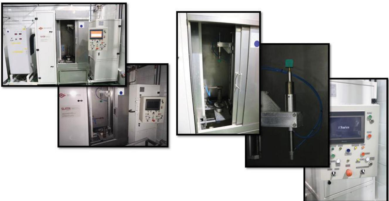
Fig. 1. HI40 induction hardening system in Research and Development Laboratory for Aerospace Materials
