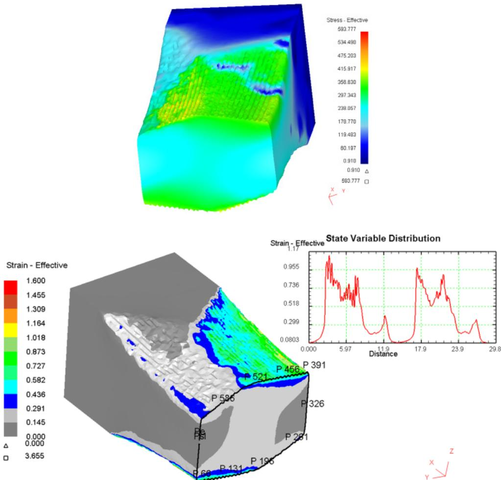
Fig. 4. Distribution intensity of stresses  $\sigma_i$  and deformations  $\epsilon_i$  in the cross-sections of the band rolled with the application of the MEFASS method (rolls having sharp-profile furrows)
