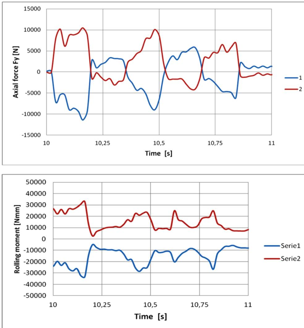
Fig. 13. Course of axial forces  $F_y$  applied to the upper (the red line, 2) and the lower roll (the blue line, 1), and also the rolling moments  $M_{w,1,2}$  in the MEFASS rolling process. Rolls having a positive curvature of a roll barrel surface
