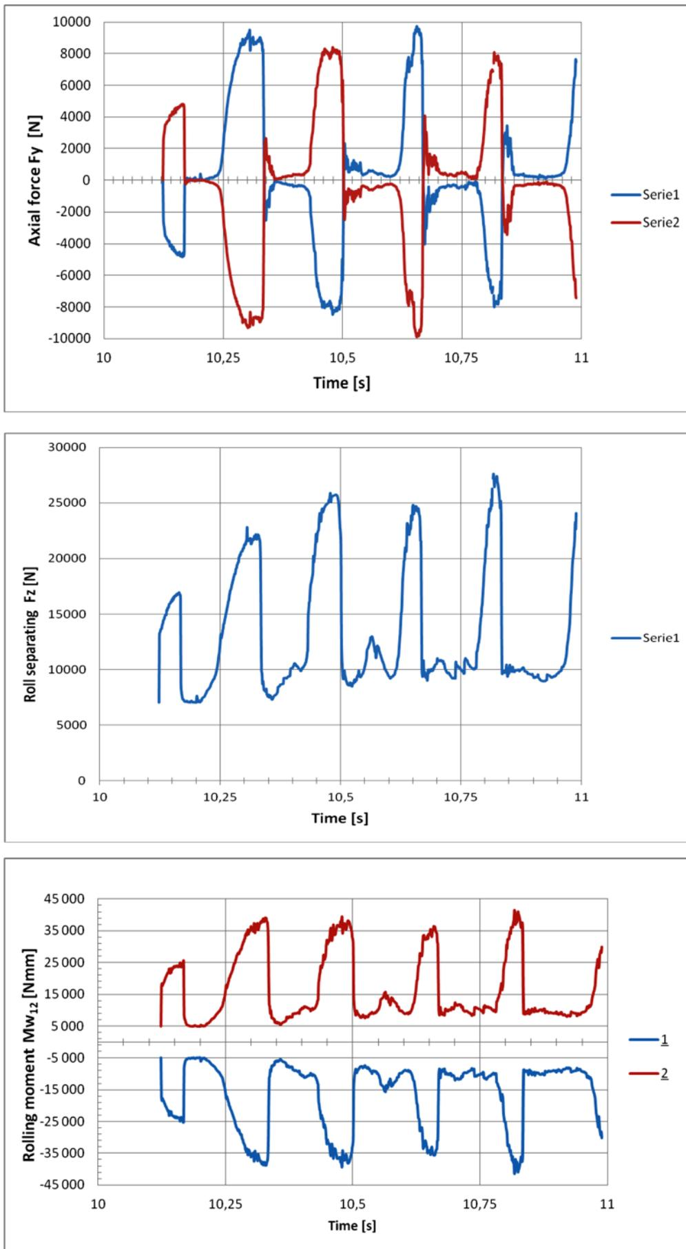
Fig. 9. Course of axial  $F_y$  and vertical  $F_z$  constituents of the rolling force acting on a roll, and also the rolling moments  $M_{w_{1,2}}$  (the upper roll – the red line, the lower roll – the blue line) in the of the MEFASS rolling process. Rolls having rounded-profile furrows
