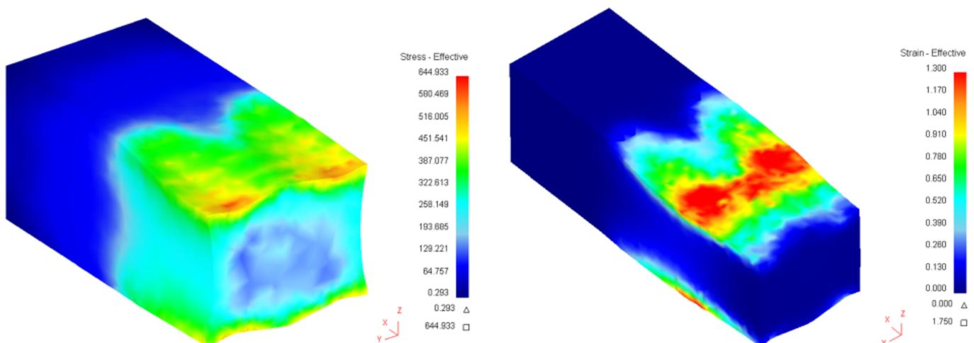
Fig. 8. Distribution intensity of stresses  $\sigma_i$  and deformations  $\varepsilon_i$  in the cross-section of the band rolled with the application of the MEFASS method – rolls having rounded-profile furrows
