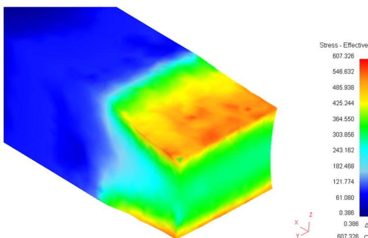
Fig. 11. Distribution intensity of stresses  $\sigma_i$  in the longitudinal cross-section of the band rolled with the application of the MEFASS method. Rolls having a positive curvature of a roll barrel surface
