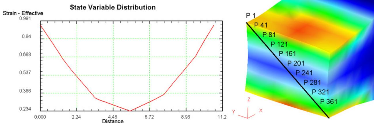
Fig. 12. Distribution intensity of deformations  $\varepsilon_i$  in the cross-section of the band rolled with the application of the MEFASS method. Rolls having a positive curvature of a roll barrel surface
