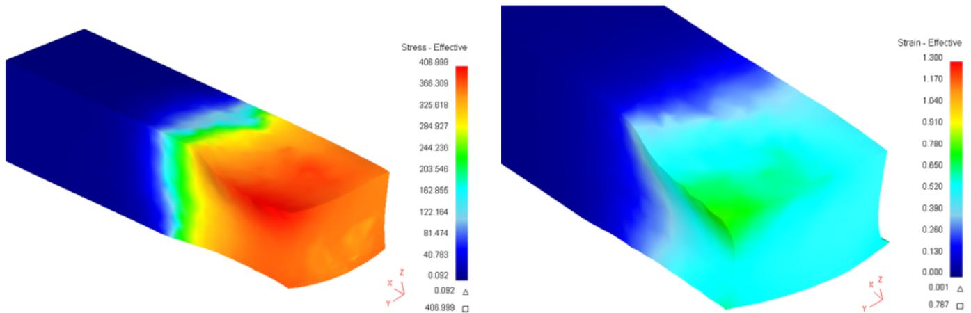
Fig. 15. Distribution intensity of stresses  $\sigma_i$  and deformations  $\varepsilon_i$  in the cross-section of the band rolled with the application of the MEFASS method. Rolls having S-profile roll barrels
