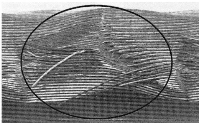
Fig. 2. Roll slip traces on a M1E copper band surface rolled in the MEFASS process
