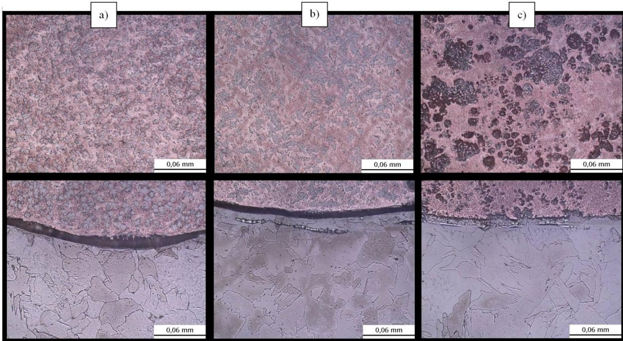
Fig. 3. Microstructure of overlay brazes (upper line) and of the area in the transition area between the overlay braze and the parent metal (lower line), made using Ar (a), Ar+1% $\text{O}_2$  (b) and Ar+18%  $\text{CO}_2$  (c), etch.  $\text{FeCl}_3$
