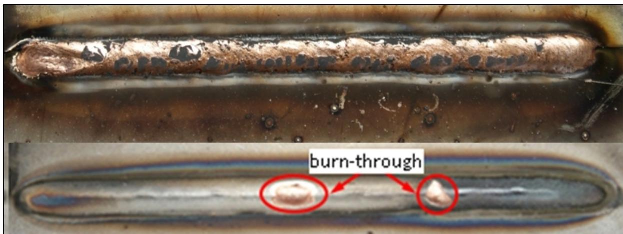
Fig. 2. Overlap joints made using various shielding gases – view of the face and opposite side of the test piece of the weldbrazed lap joints, weldbraze macrostructure (etch. Adler)
