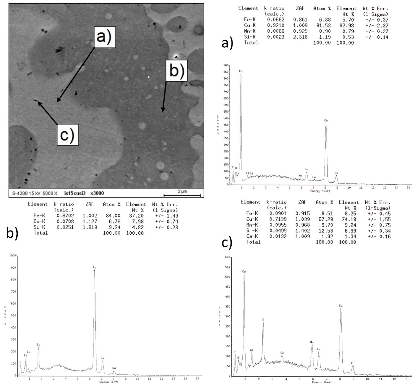
Fig. 7. Results of X-ray microanalysis of chemical composition of precipitation in transition area
