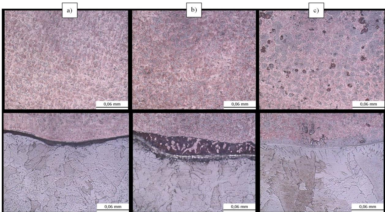
Fig. 4. Microstructure of weldbrazes (upper line) and of the area in the transition area between the weldbraze and the parent metal in the overlap joints (lower line), made using Ar (a), Ar+1% $\text{O}_2$  (b) and Ar+18%  $\text{CO}_2$  (c), etch.  $\text{FeCl}_3$
