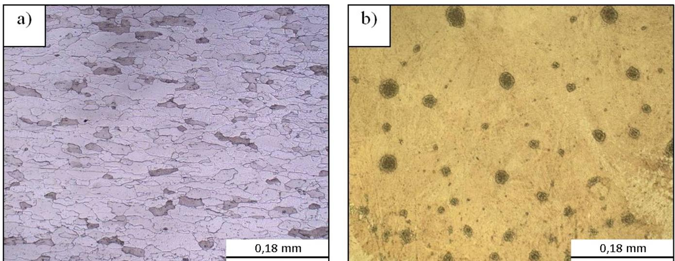
Fig. 9. Microstructure of the DC04 steel parent metal (a) and of the CuSi3Mn1 electrode wire (b), etch. FeCl<sub>3</sub>
