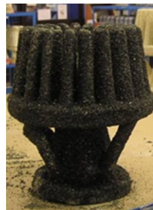
Fig. 1. The pattern assembly with 20 airfoil blade castings
