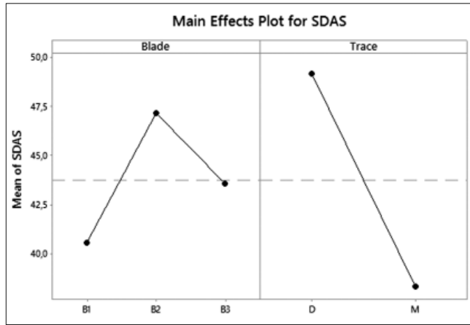
Fig. 6. The main effects plot for mean of SDAS. Blades: B1, B2, B3. Traces: D and M
