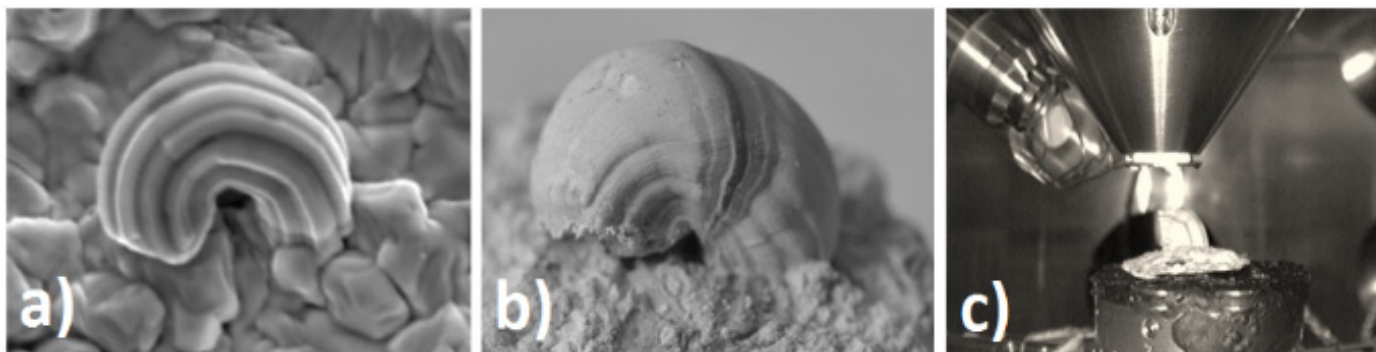
Fig. 2. 'Nodule' type whisker after the melting process – a) ~17 μm long tin whisker from literature [12] b) ~2 cm long tin-silver whisker (Sample # 4), c) Examination of a whisker in SEM
