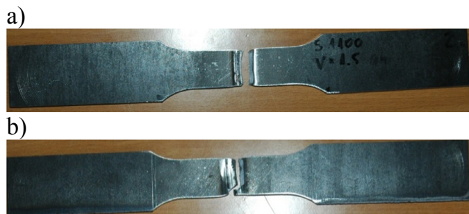
Fig. 7. A view of the broken samples from the tensile tests of butt joint A welded at 3.3 kW and welding speed of 1.5 m/min (energy input of 132 J/mm) (a) and the joint B welded at 3.3 kW and welding speed of 1.0 m/min (energy input of 198 J/mm) (b)
