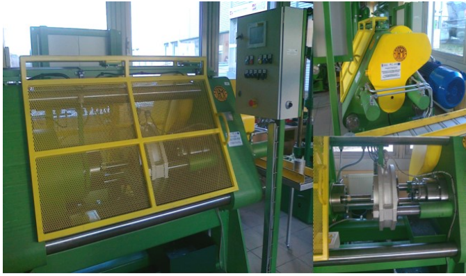
Fig. 11. Experimental KOBO press used in experiments
