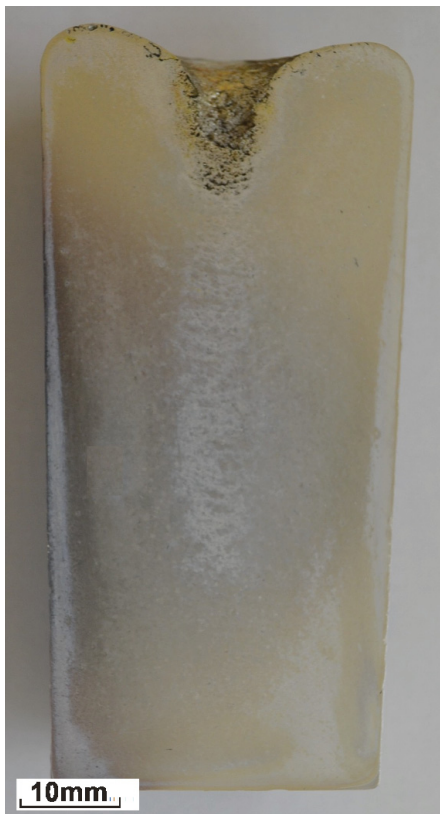
Fig. 1. Cross-section of ingot from LAZ441 alloy
