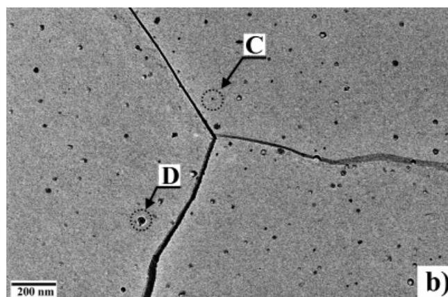
Fig. 2. Bright field TEM images of carbon extraction replicas showing the grain boundaries and distribution of secondary phase particles in SC1 (a) and SC2 (b) specimens
