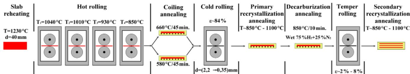
Fig. 1. Scheme of laboratory treatment of experimental steel
