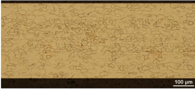
Fig. 4. The primary recrystallized microstructure of SC2 specimen after decarburization annealing at 850°C/10 min
