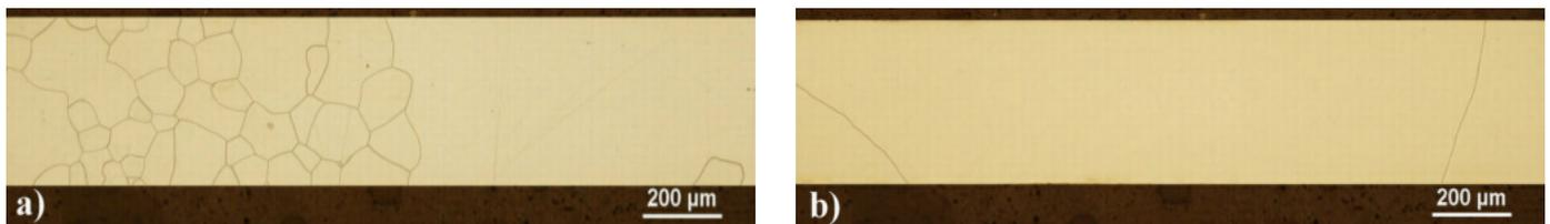
Fig. 8. The secondary recrystallized microstructure of SC2 steel after the primary recrystallization at 1075°C during 10 min, decarburising annealing, temper rolling with 4% of deformation and subsequent final annealing at dynamical conditions for 5 minutes at 1025°C (a) and 1075°C (b)
