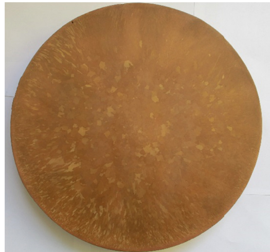
Fig. 2b. Morphology of the continuously cast brass ingot revealing columnar grains with the equiaxed (dominant) structure.
