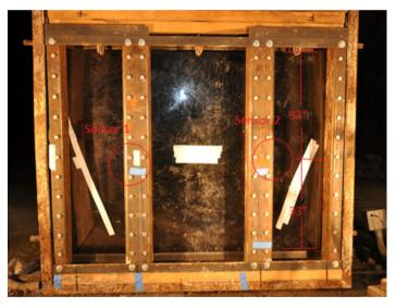
Fig. 10. Sensor Placement for Quarter-Width Scale Testing
