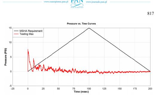
Fig. 8. MSHA Requirement Versus Half-Width Scale Measurements
