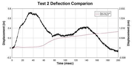
Fig. 6. Deflection Comparison of Left-Center Vertical Steel Member
