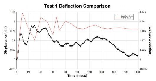
Fig. 4. Deflection at Center of the Middle Polycarbonate Panel
