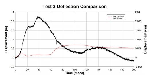
Fig. 7. Deflection Comparison of Far-Left Vertical Steel Member
