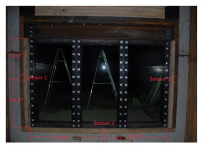
Fig. 3. Pressure Sensor Locations for Half-Width Scale Testing
