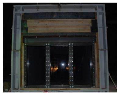
Fig. 2. Completed Half-Width Scale Polycarbonate Wall Installation
