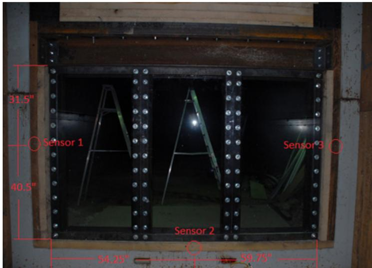
Fig. 3. Pressure Sensor Locations for Half-Width Scale Testing
