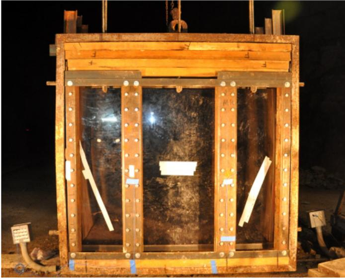
Fig. 9. Quarter-Width Scale Polycarbonate Wall System
