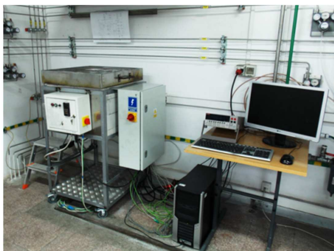
Figure 3: Experimental setup used for characterization of the 50 mm x 50 mm SOC operated as SOEC: test stand scheme (upper) and the actual photo (lower).
