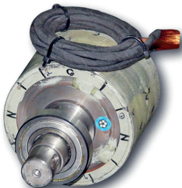
Fig. 20. Placement of the air coil on the neodymium magnet mounted on a PMSM rotor
