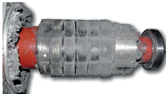
Fig. 1. The rotor of PMSM motor with damaged permanent magnets
