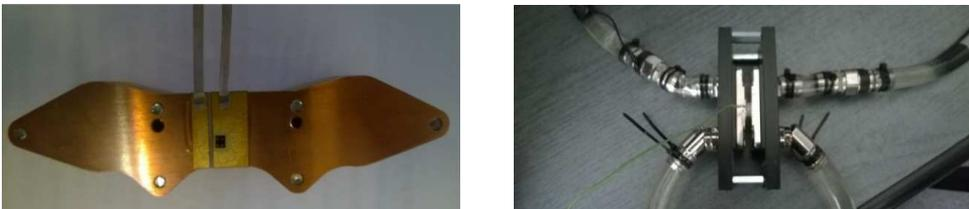
Fig. 5. Photographs of the examined diodes mounted to the liquid heat-sinks.
