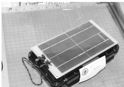
Fig. 4.1. A measurement node for monitoring water parameters (used with the permission from Prof. Prashant Shenoy).
