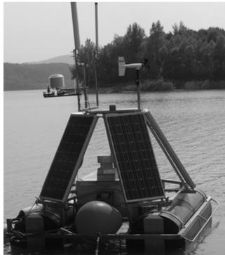
Fig. 4.2. A measurement station for monitoring the quality of drinking water.
