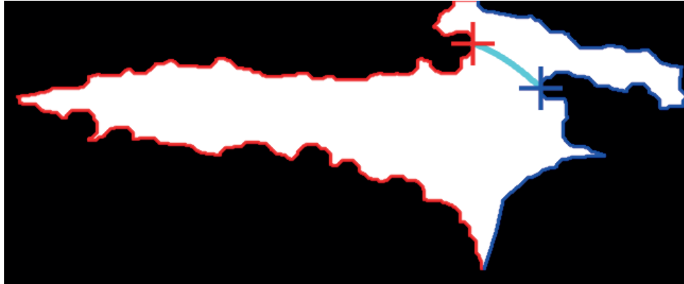
Fig. 5. Example of the division of the segmented region. The red color depicts the left profile of the blob (blue is used for the right one) and the plus sign denotes the detected local extremum in the left and right boundary of the blob transformed to 1 D. The cyan represents the line, where the blob is cut off
