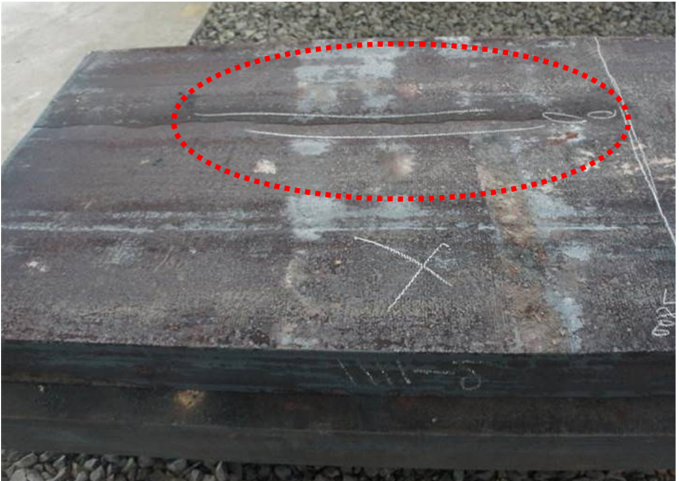
Fig. 9. A longitudinal surface crack on inside radius
