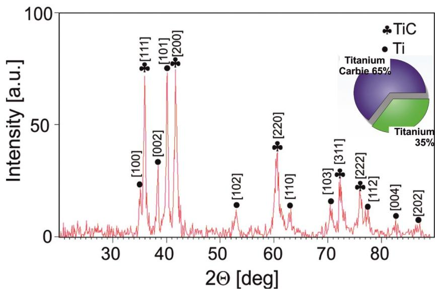
Fig. 9. X-Ray diffraction spectra of the Ti/65%TiC coating
