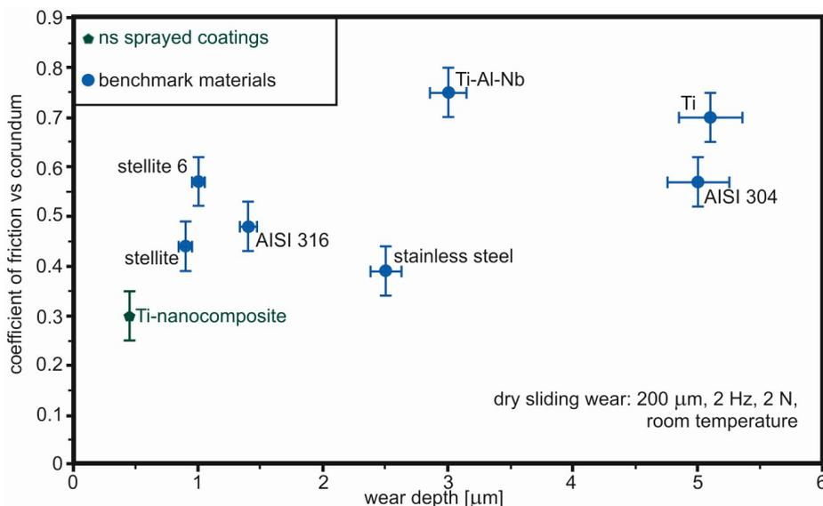
Fig. 10. Ranking of the frictional and wear characteristics of the optimal TiC/Ti nanocomposite cermets and biomedical benchmarks, obtained from pre-screening tests
