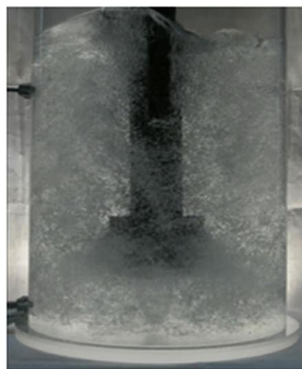
h) Variant H: 650 rpm and 10.0 Nl·min<sup>-1</sup>
