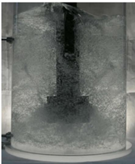
g) Variant G: 650 rpm and 5.0 Nl·min<sup>-1</sup>
