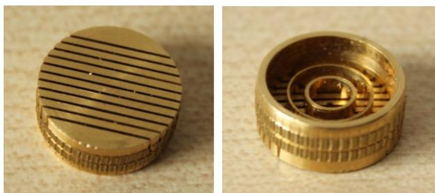
Fig. 3. Deaerating vents of the experimental core box. External diameter (for assembling) 12.15 mm, active surface 15.6 %
