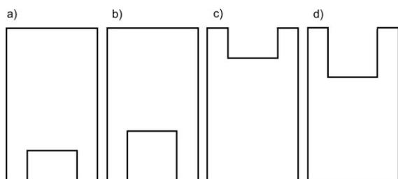
Fig. 4. Shapes of inside inserts of the horizontal experimental core box with the cuboidal cavity: a) insert with the bottom cut-out of a surface 200 mm<sup>2</sup>, b) insert with the bottom cut-out of a surface 3 cm<sup>2</sup>, c) insert with the upper cut-out of a surface 200 mm<sup>2</sup>, d) insert with the upper cut-out of a surface 300 mm<sup>2</sup>
