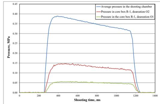
Fig. 9. Examples of the pressure pathways in the shooting chamber and the core box R-1. The shot pressure was  $0.4\text{MPa}$ , shooting hole diameter  $d = 20\text{mm}$ . Deaerations according to variants O1 and O2
