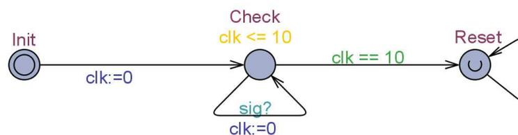
Fig. 1. Example of timed automaton – watchdog timer.
