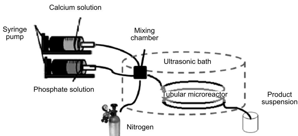
Fig. 5. Scheme of production HAp in ultrasonic tubular reactor. Reprinted from (Castro et al., 2013a) with permission from Elsevier (Copyright 2013)
