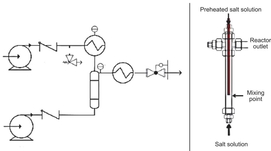
Fig. 2. Scheme of continuous hydrothermal synthesis (left) and hydrothermal rig (right). Reprinted from (Lester et al., 2012) with permission from Elsevier (Copyright, 2011)
