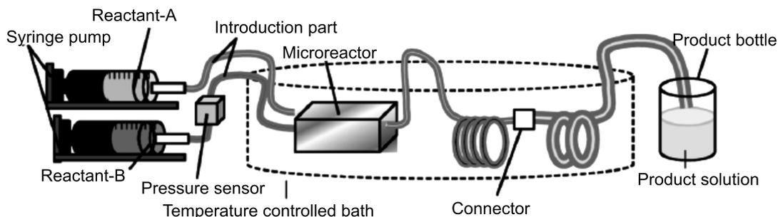
Fig. 4. Scheme of microsystem reactor. Adapted from (Kandori et al., 2011) with permission from American Chemical Society (Copyright, 2011)
