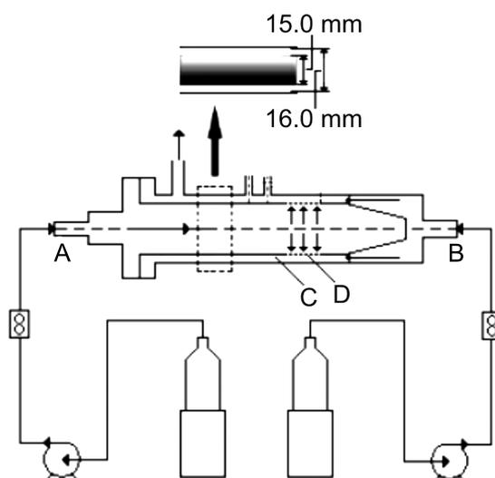
Fig. 3. Scheme of tube-in-tube microchannel reactor. A-inlet of inner tube; B-inlet of outer tube; C-microchannel; D-micropores. Adapted from (Yang et al., 2010) with permission from American Chemical Society (Copyright, 2010)
