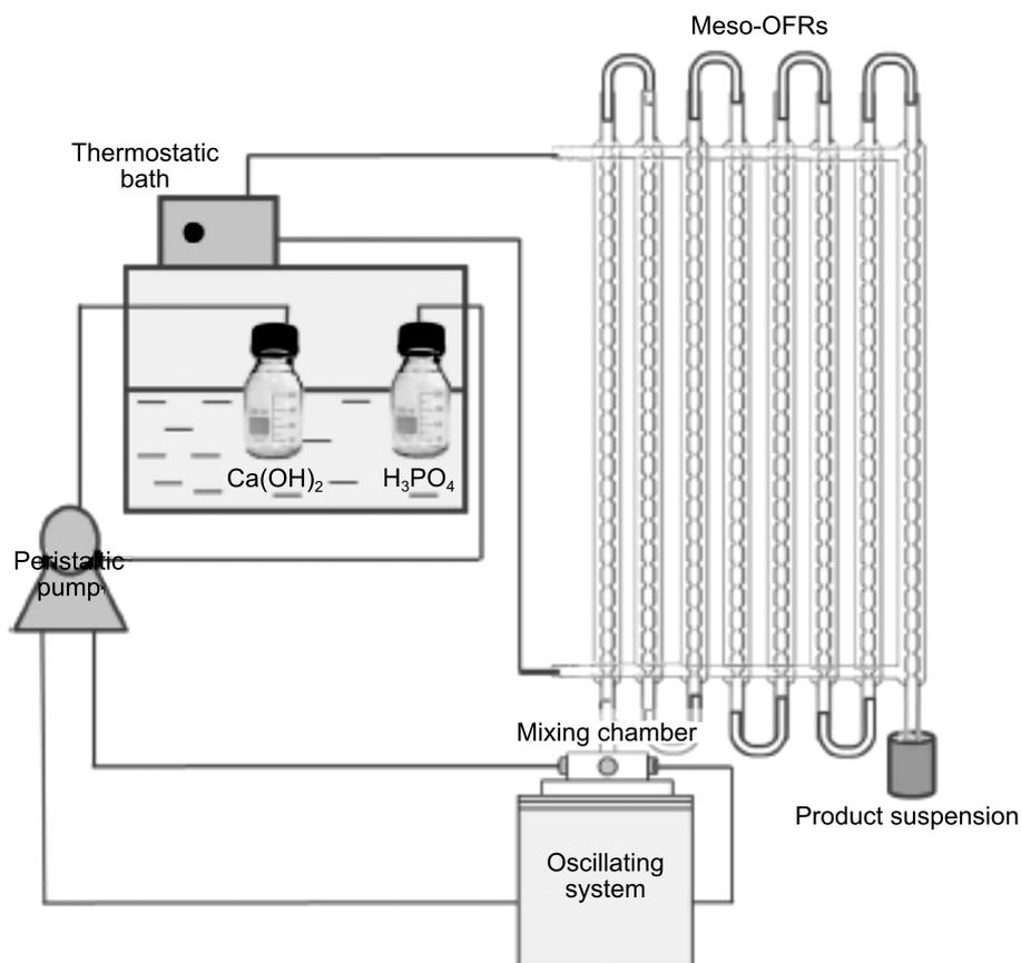
Fig. 6. Scheme of HAP production in scaled-up meso-OFR. Adapted from (Castro et al., 2013b) with permission from American Chemical Society (Copyright, 2013)
