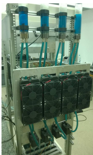
Fig. 6. A hydraulic circuit of the heat exchanger.
