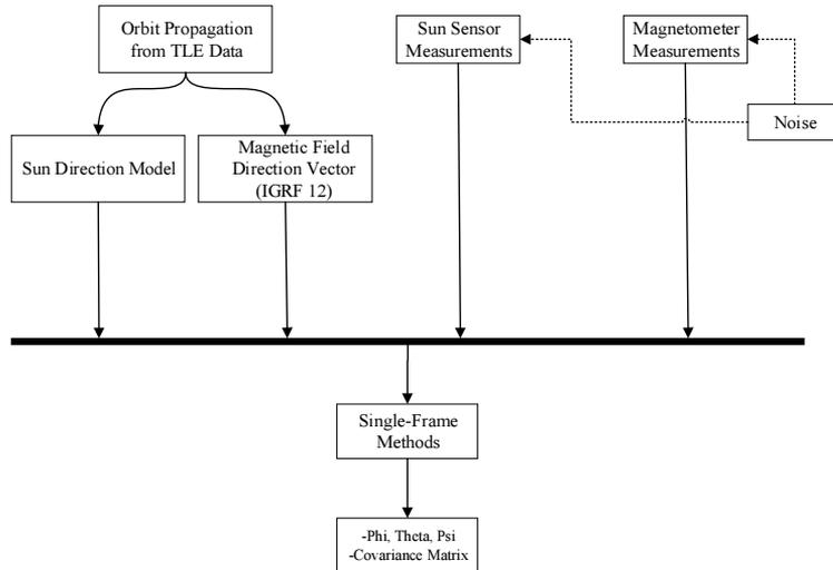
Fig. 1. A block diagram of the Sun and Earth’s magnetic field vectors-based single-frame attitude determination methods.
