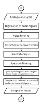
Fig. 1. Flowchart of a standard analysis algorithm of a voice signal
