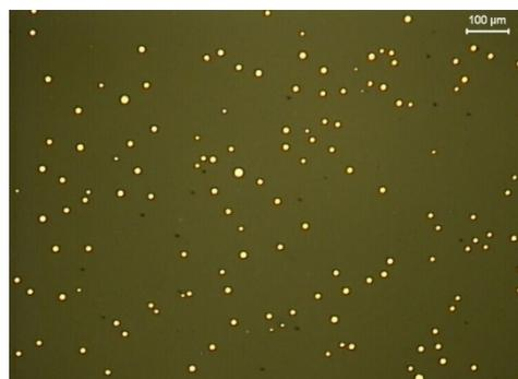
Fig. 5. Agglomeration and coagulation of the droplets in the slag
