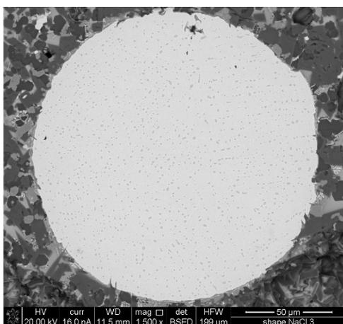
Fig. 2. Fully spherical coagulated droplet which contain about 85 wt.% Cu and some precipitates of the Cu-Cu<sub>2</sub>O – eutectic [7]
