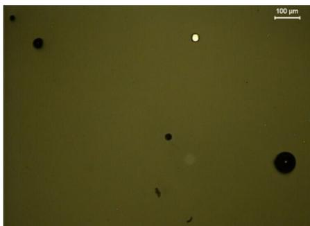
Fig. 8. Remaining, well coagulated individual copper droplet in the cooled slag after treatment by the patented, complex reagent with the small addition of  $\text{Na}_2\text{CO}_3$
