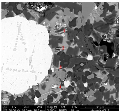
Fig. 1. Copper droplets shape; a/ (1,2,3,4 - rods) - containing below 15 wt.% Cu tend towards the main copper droplet, b/ main / large copper droplet (irregular in shape) in the course of coagulation [7]
