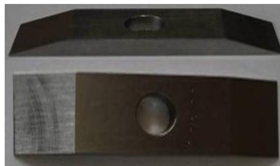
Fig. 2. Sample for evaluation of the resistance to thermal shocks
