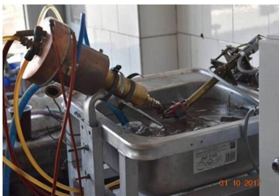
Fig. 1. A device for simulating heat shock
