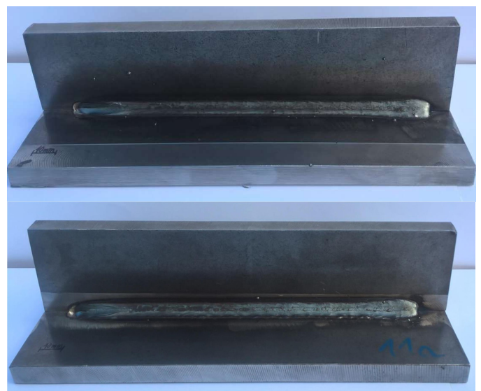
Fig. 5. T-joint welded double-sided welding technique LA
