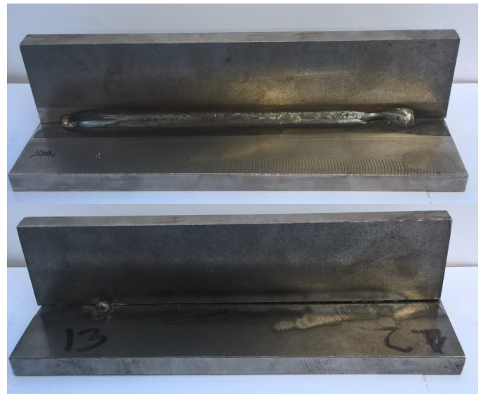
Fig. 4. T-joint one-sided welding technique LA
