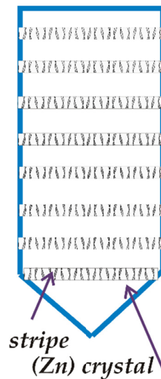
Fig. 7. Schematic outline of a single crystal decorated with stripes (strengthening layers) of constant spacing and width, and the morphology relevant to an imposed growth rate
