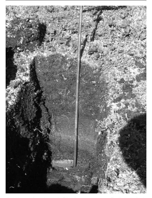
Fig. 4. The excavation made on the Storflaket mire near ERT surveys profile (Fig. 2), showing the base of the active layer at a depth of c. 80 cm.
