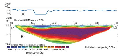
Fig. 3. **A.** Active layer depth as measured by using a steel rod. **B.** Results of the deep ERT-surveys profiling in the same locality as in Fig. 2, with different electrode spacing. The active layer connot be identified.
