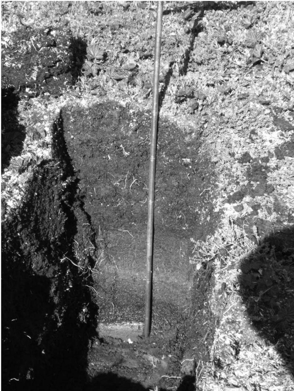
Fig. 4. The excavation made on the Storflaket mire near ERT surveys profile (Fig. 2), showing the base of the active layer at a depth of *c.* 80 cm.
