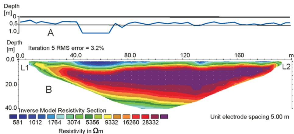
Fig. 3. **A.** Active layer depth as measured by using a steel rod. **B.** Results of the deep ERT-surveys profiling in the same locality as in Fig. 2, with different electrode spacing. The active layer cannot be identified.
